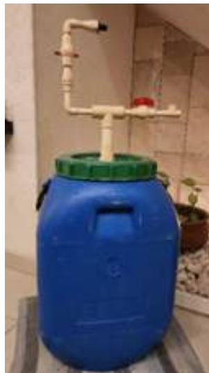
Fig. 1. Bioreactor with CPVC biogas transport pipes - Own elaboration.
