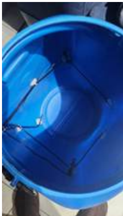
Fig. 7. Instrumentation of pH and temperature sensors in biodigester - Own elaboration.
