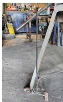
Fig. 6. Construction of the paddle agitator in a blacksmith workshop - Own elaboration
