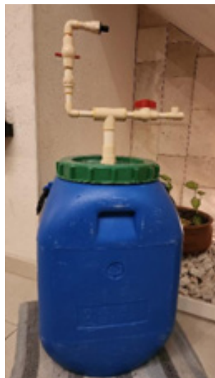
Fig. 1. Bioreactor with CPVC biogas transport pipes - Own elaboration.
