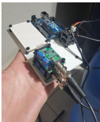
Fig. 8. Control board for sensor instrumentation in biogestor - Own elaboration.
